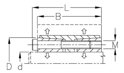
B mm = 155d H8 mm = 380D mm = 475Fit tolerance = Aksel h8, Nav H8 F kN torque = 2784.0L mm = 177M mm = M22P N/mm2 surface pressure on shaft/hub = 135 Surface roughness = R? ?  $3.2 \mu n$ T N m torque = 529000Ts N m bolt tightening torque = 930.0
